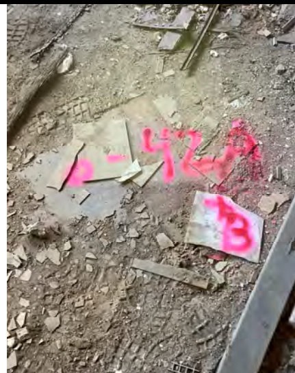
Sample # 42 Flooring - 9X9 Floor Tile with Glue- Beige
