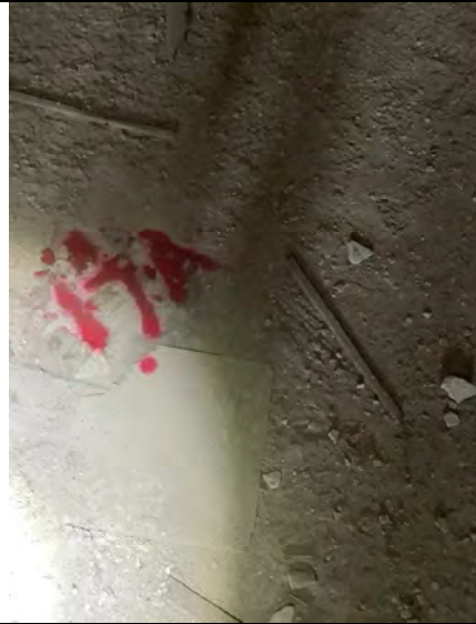
Sample # 17 Flooring - 12X12 Floor Tile with Glue- White with Mosaic pattern
